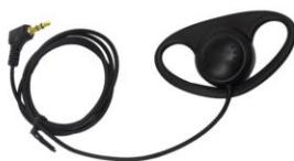
Mono earphone compatible with TG 100RX receivers. Thanks to its shape it is easy to wear and it is particularly lightweight and almost imperceptible. It is ideal for guided tours, conferences etc.. Impedance: 32 Ohms, speaker: 27mm, sensitivity: 105db, freq response: 20hz-20khz, max input power: 80mW. Stereo jack
