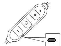
Connect the supplied cable to the indicated port and then to a standard USB socket. Charging time is of about 2 hours and the solid blue led shows it is completed.
