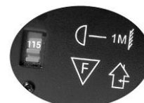
Figure 1 - AC Voltage Switch
