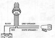
The output impedance of this set is automatically adjusted to 4-16 ohms, therehore, any speaker, 4-16 ohms, can be connected.
