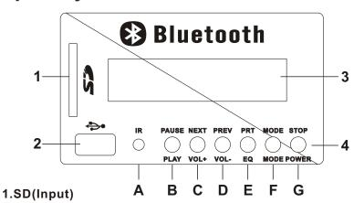
This slot is used to insert a SD, non-volatile memory card with Mp3 files to be read.
